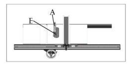
2. Adjust the rip fence (A) according to material size and place the magnetic base to the right of the feed direction (B). Before placing the base, check that the locking screw is extended.
