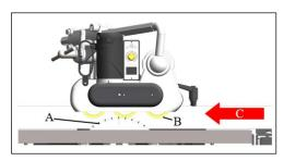
**3.** To feed the material correctly, the distance between the infeed roller (B) and fence should be 3-5 mm greater than the distance between outfeed roller (A) and fence.
