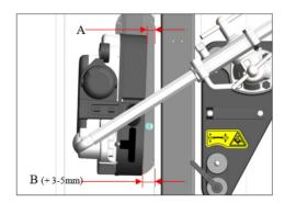
4. Lower the blade into the table and check that all rollers are in contact with the material. This will ensure smooth feeding. Do not exert too much pressure on the material, it may cause the base to shift.
