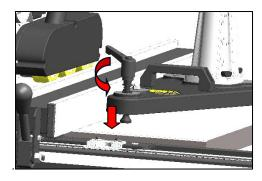
**4.** Adjust feeder position so that feed rollers (B) are between the blade (A) and the rip fence (C).
