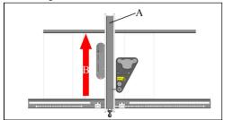
3. After placing the base in a suitable spot, rotate the locking handle until the locking screw is completely retracted. Check by hand that the base is securely attached.
