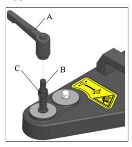
**3**. Rotate the locking handle (A) to protrude the locking screw (B). Now move the base to a suitable spot.
