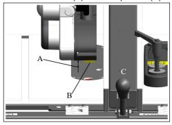
5. The feed roller should extend beyond the saw blade edge at the feed entry (C). The material must first touch the roller (B), then the blade (A).
