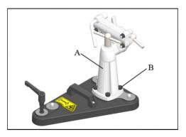
5. Grab the feeder arm (A) and handle on the base (B). Move the base with mounted feeder.
