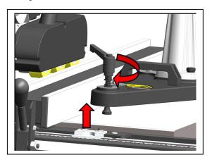
**9**. Grab the feeder arm (A) and handle on the base (B). Move the base with mounted feeder.
